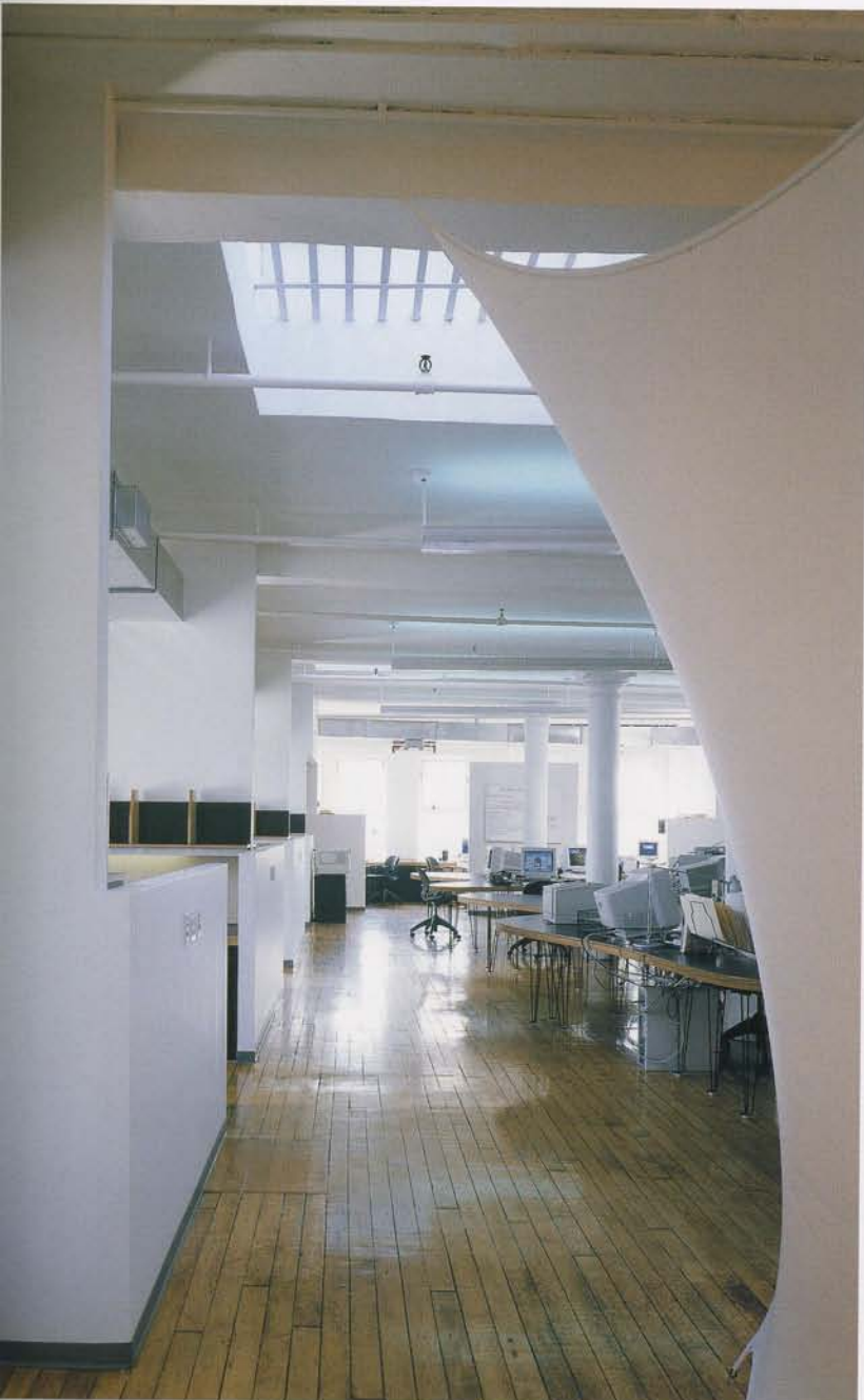
⊗ Low-acrylic partitions measuring four-, five-, or seven-feet (1.2, 1.5, or 2.1-meter) high, create an envelope wrapping the perimeter that define semiprivate offices for the creative team.
